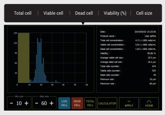
EVE™ PLUS measures the number and concentration of total cells, viable cells, dead cells. It provides viability results and cell size gating.
