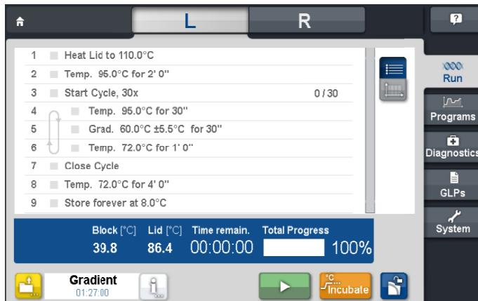
Note: With the VWR Doppio double block thermal cyclers the desired block can be chosen by selecting 'L' (left) and 'R' (right). This option is not available for the VWR UNO<sup>96</sup>, UNO<sup>384</sup> and Ristretto.
