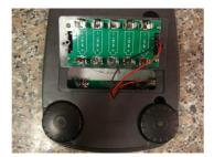
3. Insert five AA 1,5V batteries taking care of the right position of each battery.
