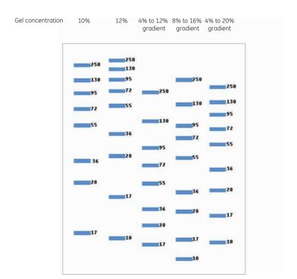
**Fig 3.3.** When selecting a gel, it is important to use an acrylamide concentration that will allow optimal separation of the proteins in your sample. High molecular weight proteins will be optimally resolved in gels containing a lower acrylamide content, while smaller proteins should ideally be run in more acrylamide-dense gels. The image shows the separation pattern for nine different proteins for each acrylamide concentration.
