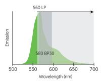
**Fig 7.3.** Emission filtering of Cy3 fluorescence using either a 580 BP30 filter (dark-gray area) or a 560 LP filter (light- and dark-grey areas). BP = band pass. LP = long pass.
