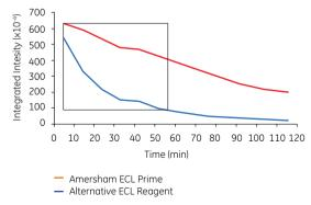
**Fig 6.7.** Signal stability over time. The signal duration of Amersham ECL Prime compared to an alternative chemiluminescent detection reagent. The high stability of Amersham ECL Prime provides a broader window of time in which higher sensitivity is maintained.
