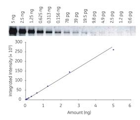
**Fig 6.13.** Fluorescence detection with Amersham ECL Plex gives a broad linear dynamic range, making it possible to detect and compare weak and strong bands on the same blot. This is a dilution series of transferrin detected with Cy3-labeled secondary antibodies. The dynamic range is 3.6 orders of magnitude and very linear with an LOD of 1.2 pg.
