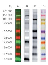
Fig 3.7. Amersham ECL Plex Fluorescent Rainbow Markers imaged on a Typhoon scanner. From left to right: (A) Full-color Cy3 and Cy5; (B) Cy3 channel; (C) Cy5 channel; and (D) visible spectrum.
