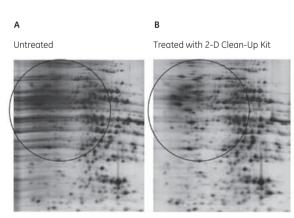
Fig 2.2. 2-D Clean-Up Kit eliminates most of the horizontal streaking caused by residual SDS. Sample: Rat liver extracted with 4% SDS, 40 mM Tris base. First dimension: Approximately 20  $\mu$ g of rat liver protein, Immobiline<sup>TM</sup> DryStrip (pH 4–7, 7 cm). Ettan<sup>TM</sup> IPGphor<sup>TM</sup> 3 Isoelectric Focusing Unit unit 17.5 kVh. Second dimension: SDS-PAGE (12.5%), run on SE 260 Mini-Vertical Unit (8  $\times$  9 cm gel). Stain: PlusOne Silver Staining Kit, Protein.
