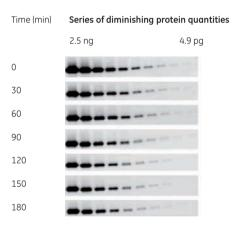
**Fig 8.3.** Amersham ECL Prime signal duration is monitored for 3 h after the addition of reagent by capturing images every 30 min with the same exposure time of 3 min. The majority of the bands are still detectable, and allow precise quantitation even after 3 h.
