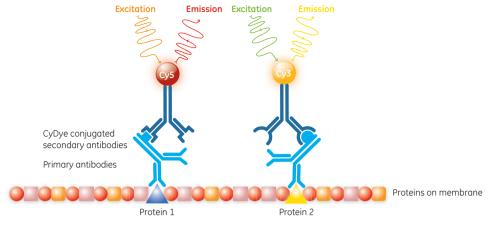
**Fig 6.12.** The principle of Amersham ECL Plex. Primary antibodies against two proteins are recognized by species-specific secondary antibodies conjugated to fluorescent CyDye, Cy3 and Cy5. Detection by direct fluorescence reduces the number of processing and imaging steps, which saves time and reduces errors in quantitation.
