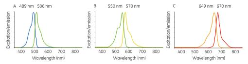
**Fig 6.11.** Excitation and emission spectra for fluorescent CyDye (A) Cy2, (B) Cy3, and (C) Cy5. In each example, the effect of the light wavelength generating the maximum efficiency of excitation is shown.
