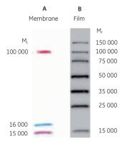
Fig 3.6. Amersham ECL DualVue Western Blotting Markers after electrophoresis on a 4% to 20% SDS gel and transfer onto an Amersham Hybond<sup>TM</sup> ECL nitrocellulose membrane (now replaced by Amersham Protran<sup>TM</sup> Premium 0.45 nitrocellulose blotting membrane). Prestained indicator proteins are shown as a photograph of the membrane (A), together with tagged recombinant proteins after detection with Amersham ECL as a photograph of the film, following 1 min exposure (B).
