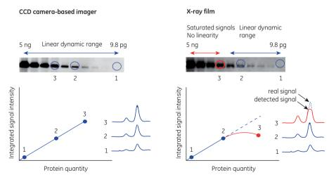
Fig 8.2. The advantage of using a CCD camera-based imager compared to X-ray film for signal detection. For the CCD camera-based system, all bands fall within the linear dynamic range of the system, whereas for film, the most intense bands (indicating more protein) are saturated, rendering quantitation impossible at this portion of the curve as the volume under the curve can no longer be determined.
