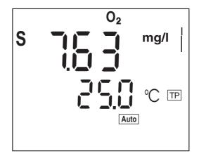
2 To terminate the Hold function: press the **<MODE>** or **<HOLD>** key. The S in front of the measured value is no longer displayed.
