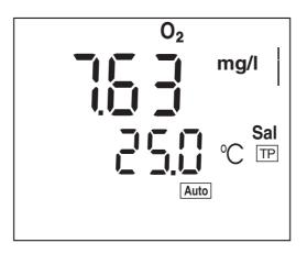
2 Switch off the salinity correction with  $\langle \nabla \rangle$ . The SAL display indicator is no longer displayed.
