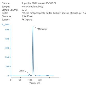
Fig 4.4. Separation of the monomer and dimer of a monoclonal antibody on Superdex 200 Increase 10/300 GL.
