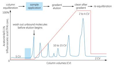
Fig A9.8. Typical RPC gradient elution.
