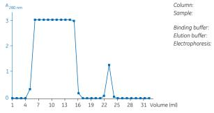
HiTrap Protein G HP 1 ml 10 ml cell supernatant containing mouse monoclonal IgG<sub>1</sub>, anti-transferrin 20 mM sodium phosphate, pH 7.0 100 mM glycine-HCl, pH 2.7 SDS-PAGE, PhastSystem, PhastGel Gradient 10–15, 1 µl sample, silver stained
