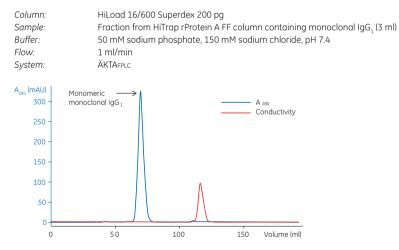
Fig 6.3. Polishing on HiLoad 16/600 Superdex 200 pg.
