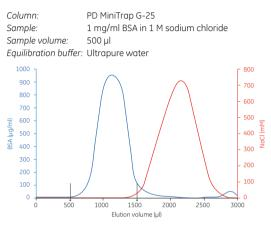
Fig 2.12. Removal of sodium chloride from BSA using the gravity protocol. The protein recovery was 95%.
