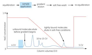
Fig A9.5. Typical HIC gradient elution.
