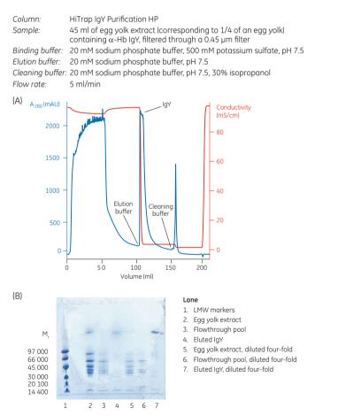
Fig 3.34. (A) Purification of IgY on HiTrap IgY Purification HP. (B) SDS-PAGE of nonreduced samples on PhastSystem using PhastGel 4–15, Coomassie staining.
