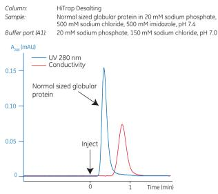
Fig 2.5. Typical desalting of a normal sized globular protein using a chromatography system.
