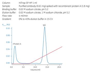
**Fig 4.5.** Removal of protein A from mouse IgG<sub>2b</sub> by cation exchange chromatography on HiTrap SP HP. Recombinant protein A was spiked into mouse IgG<sub>2b</sub> previously purified on rProtein A Sepharose Fast Flow.
