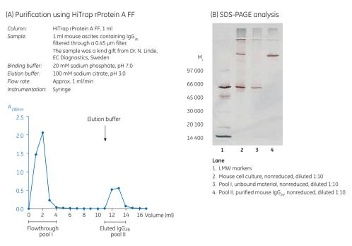
**Fig 3.21.** (A) Purification of mouse IgG<sub>2b</sub> from ascites on a 1 ml HiTrap rProtein A FF column using a syringe. (B) Analysis of eluted IgG<sub>2b</sub> by SDS-PAGE on PhastSystem and a PhastGel Gradient 10-15 precast gel revealed a purity of 95% (silver staining).
