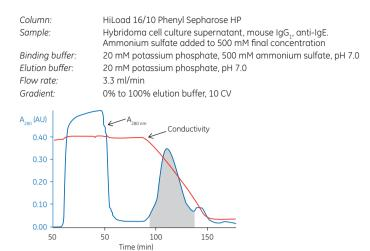
Fig 6.9. Capture of mouse IgG, on HiLoad 16/10 Phenyl Sepharose HP.
