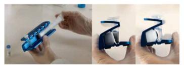
Fig 3.27. The high density of Mag Sepharose beads allows rapid capture by MagRack 6 magnetic device.
