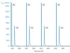
Fig 6.8. Chromatogram of four repetitive runs showing purification of human monoclonal antibody from cell culture by affinity chromatography (AC) and desalting (DS).
