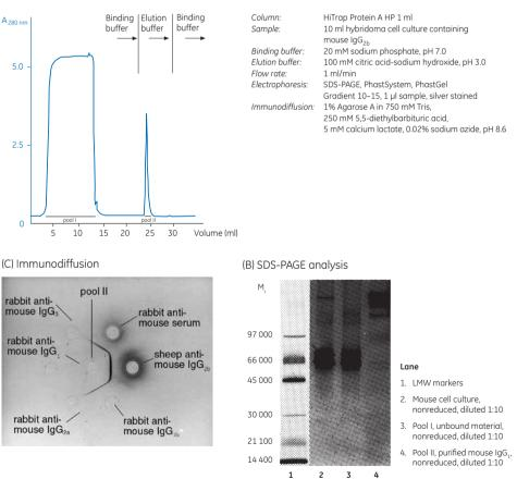
**Fig 3.18.** (A) Purification of mouse monoclonal IgG<sub>2b</sub> from cell culture supernatant on HiTrap Protein A HP, 1 ml column. Purity of mouse IgG<sub>2b</sub> was confirmed by (B) nonreducing SDS-PAGE on PhastSystem using PhastGel 10-15 (silver stained), and (C) agarose-gel immunodiffusion.
