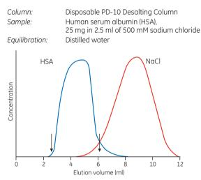
**Fig 2.14.** Removal of sodium chloride from albumin solution. A PD-10 Desalting column was equilibrated with distilled water. The sample contained human serum albumin (25 mg) dissolved in 2.5 ml of 500 mM sodium chloride solution. A total of 23.8 mg albumin was recovered in 3.5 ml eluent corresponding to a yield of 95.3% (between arrows). Initial total salt content of sample before desalting was 2%.
