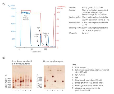
Fig 3.33. (A) Purification of α -Shigella IgM on HiTrap IgM Purification HP. (B) SDS-PAGE of sample, flowthrough, and eluted pools was performed under reducing (left gel) and nonreducing (right gel) conditions. SDS-PAGE was performed on PhastSystem using PhastGel 4–15, silver staining.
