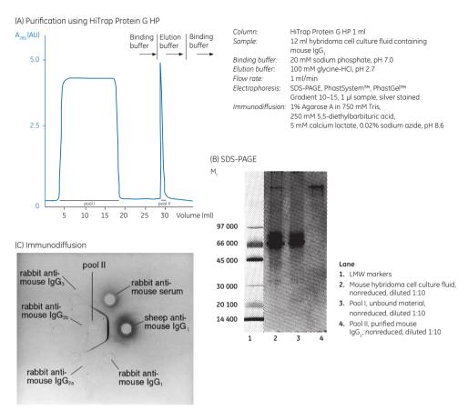
**Fig 3.11.** (A) Purification of mouse monoclonal IgG<sub>1</sub> from cell culture supernatant on HiTrap Protein G HP 1 ml column. Purity of mouse IgG<sub>1</sub> was confirmed by (B) nonreducing SDS-PAGE on PhastSystem using PhastGel 10-15 (silver stained), and (C) agarose-gel immunodiffusion.
