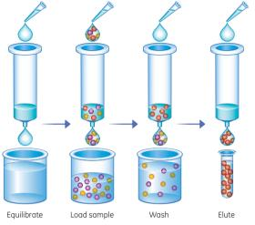
Fig 3.5. Purifying antibodies withProtein G GraviTrap is a simple four-step procedure.
