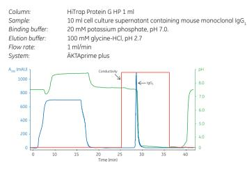
**Fig 6.5.** Capture step in a two-step purification of mouse monoclonal IgG<sub>1</sub> using HiTrap Protein G HP. The curves shown are absorbance (blue), pH (green), and conductivity (red).
