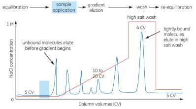
Fig A9.2. Typical IEX gradient elution.
