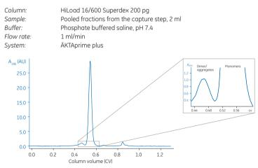
Fig 6.6. Note the separation between dimers and monomers (magnified).
