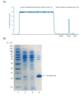
Fig 3.31. (A) Purification of Dab fragments from *E. coli* using Capto L. (B) SDS-PAGE under reducing conditions of sample load, flowthrough, and eluted fractions from the purification of Dab fragments on Capto L. SDS-PAGE was run under reducing conditions, Coomassie staining.
