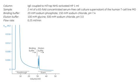
Fig 3.35. Purification of an IgE-stimulating factor from a human T-cell line.
