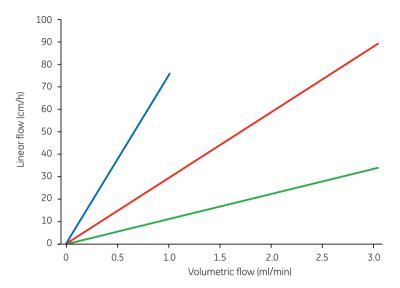
Fig A7.1. Linear flow as a function of volumetric flow: Blue curve 10 mm, red curve 16 mm, and green curve 26 mm column diameter.
